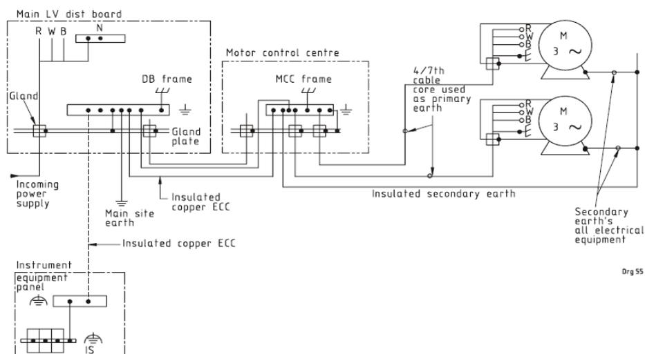
Figure 4: Earthing and bonding of electrical circuits
