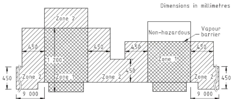
**Figure 2: Hazardous locations associated with typical dispensers**
