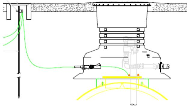
**Figure 6: Earthing and bonding of a metal filler box**
