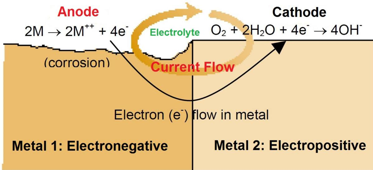
Figure 1: Corrosion cell / bimetallic corrosion
