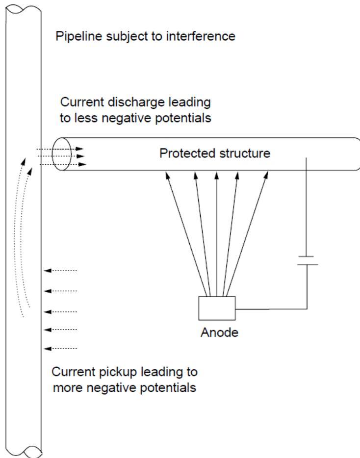
**Figure 14: Cathodic interference example**
