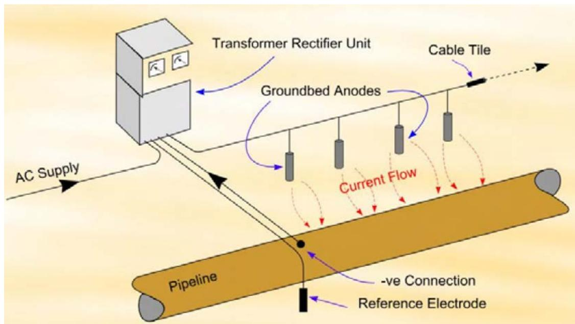
**Figure 7: ICCP Typical application on a pipeline**
