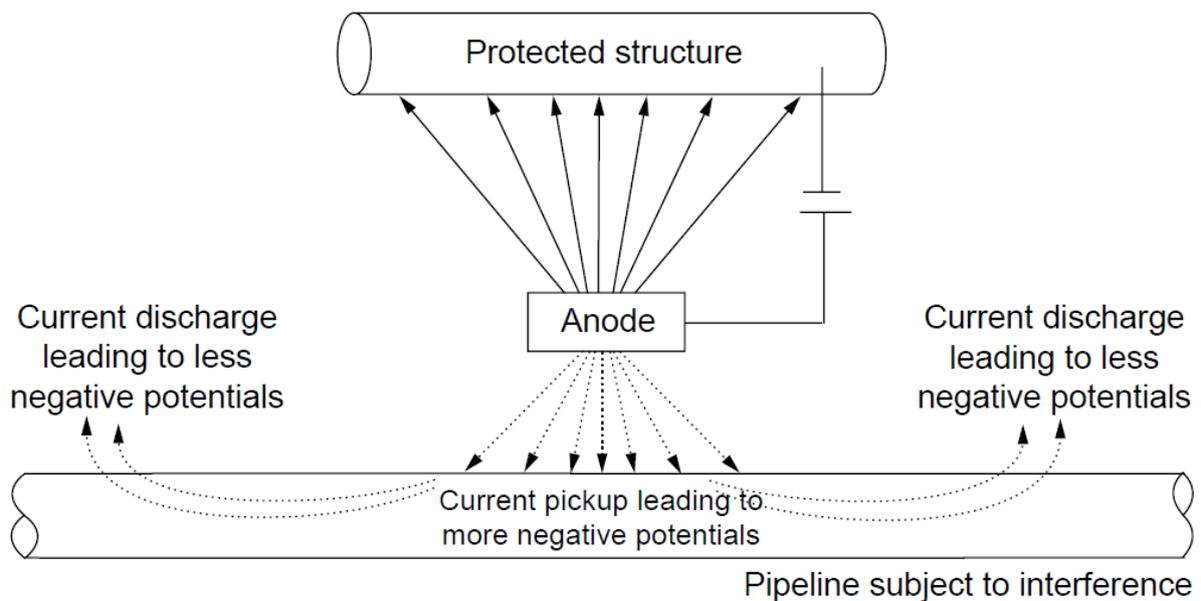
**Figure 13: Anodic Interference Example**
