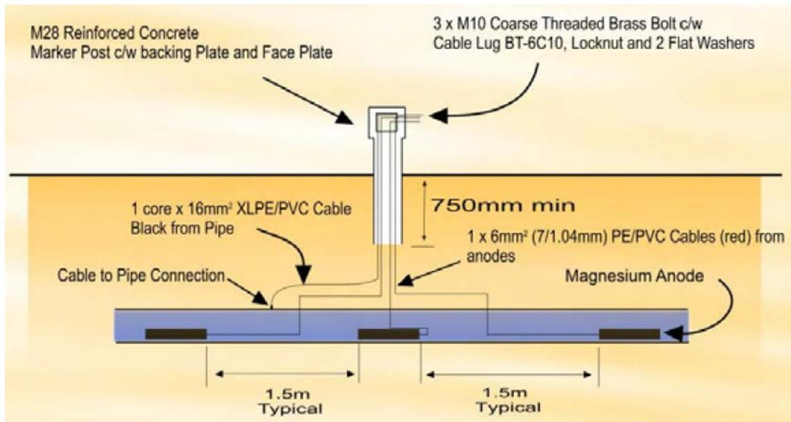
**Figure 5: SACP Typical application on a pipeline**
