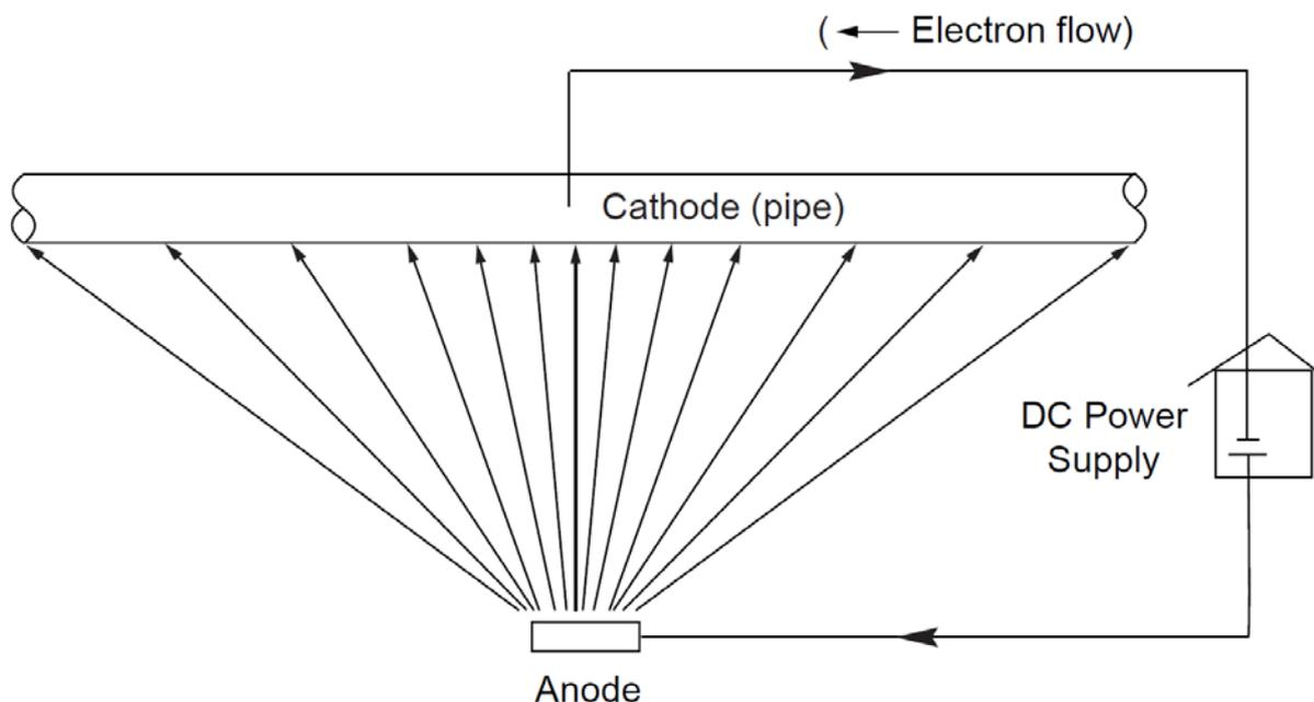
Figure 2: Basic ICCP Diagram
