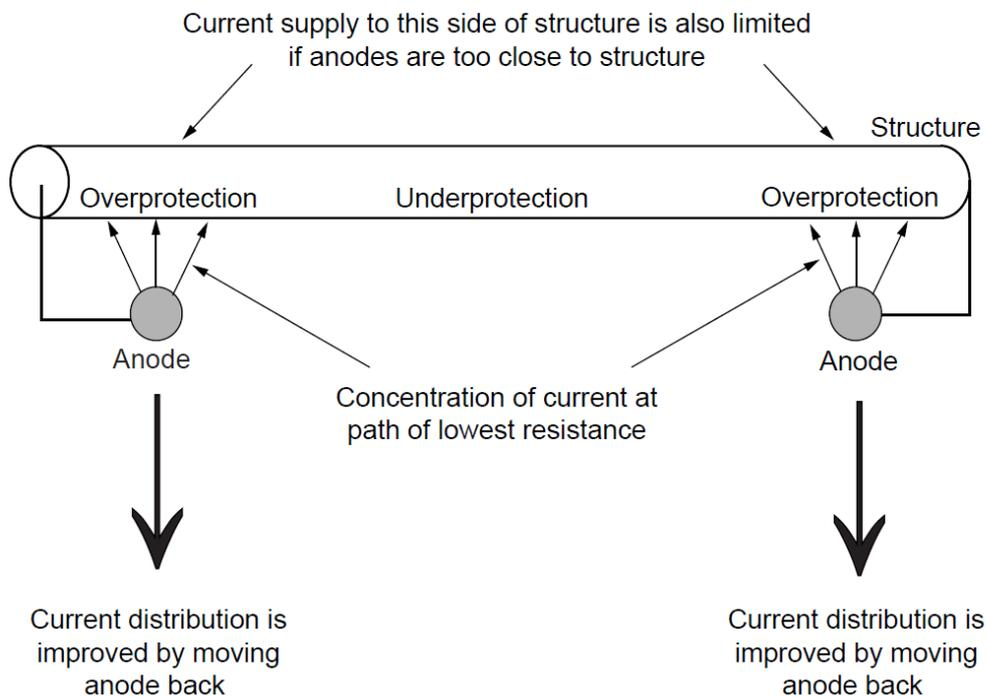
**Figure 11: Anode Layout**
