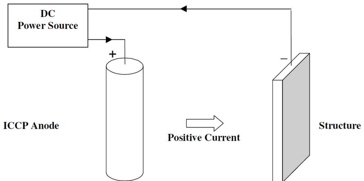
**Figure 6: Impressed Current Cathodic Protection (ICCP)**
