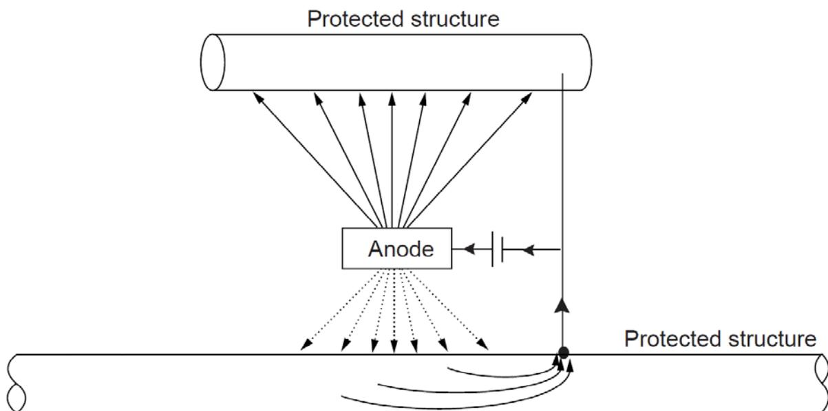
**Figure 16: Drainage bond to mitigate stray current**
