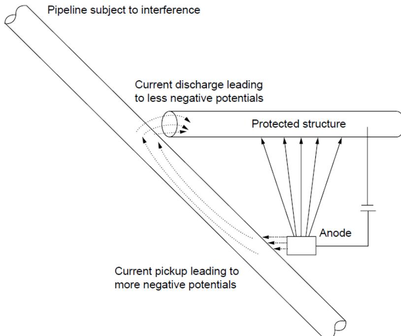
**Figure 15: Combined anodic and cathodic interference example**
