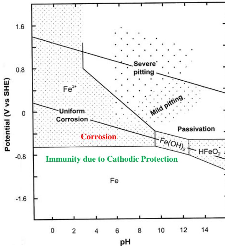
Figure 8: Stability Diagram for Iron
