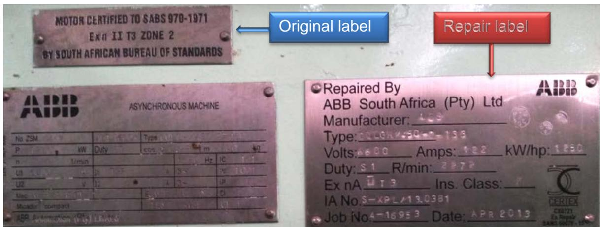
Figure 3: Original and repair label on Ex nA motor
