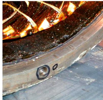
Figure 5 : Flame path scratch
