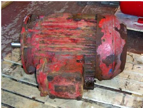
Figure 1 : Ex d motor before repair
