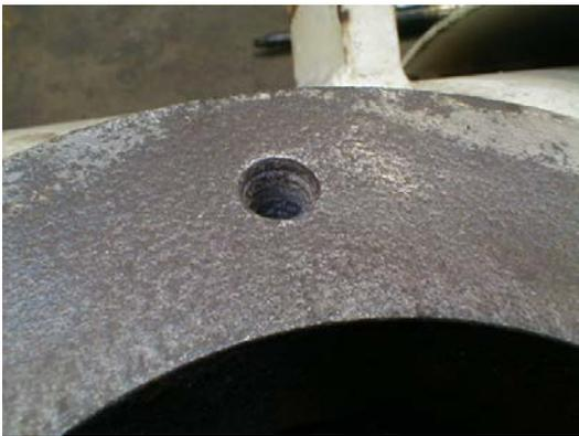
Figure 4: Corroded flange face and threaded hole on face
