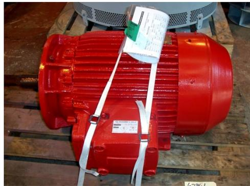
Figure 2 : Ex d motor after repair
